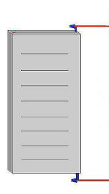
Conventional radiators are designed to deliver useful heat at temperatures of no less than 80degC
