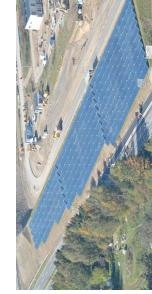
Hillerød Forsyning uses a DH scheme to supply 15000 houses using 80% gas CCGT CHP, 4% gas boilers, 14% wood pellet boilers and 2% solar thermal fields.
