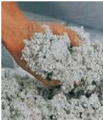
Cellulose: 0,040 W/m·K (10% Borax, fireprotection and fungicide)
