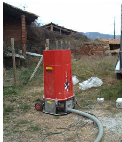
Cellulose: 0,040 W/m·K (10% Borax, fireprotection and fungicide)
